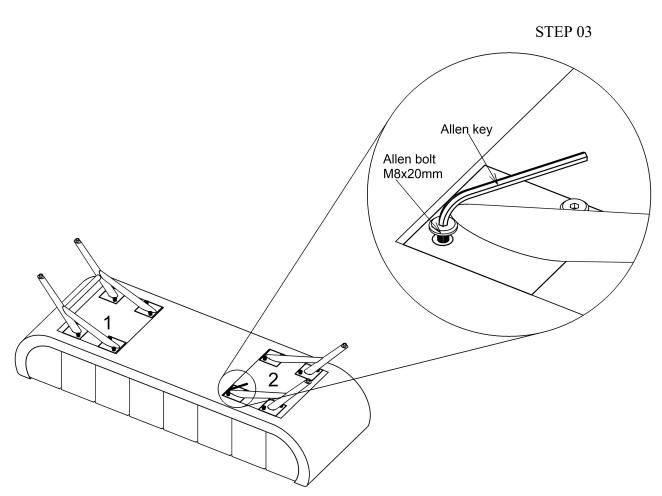
Fix the Part-A & Part-B(2) with using Allen bolt M8x20mm with help of Allen key at position 2 as shown in Fig.
