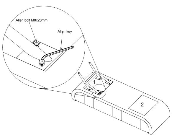
Fix the Part-A & Part-B(1) with using Allen bolt M8x20mm with help of Allen key at position 1 as shown in Fig.
